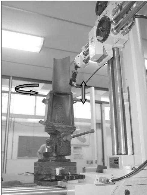
**Figure 1.** First stage air cooled blade measurement. Arrows indicate the MMC sensor displacement on the blade.
